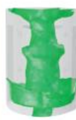
Contours of Mass fraction of tracer (Time = 1.3000e+01) Mixing time calculation
